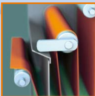
1 Pneumatisch geregelte Pendelwalze Pneumatically controlled compensator rollers
